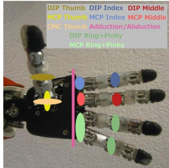
Figure 1 - Kinematic structure of the hand of the iCub
