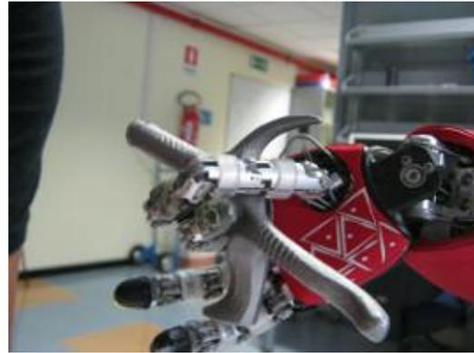
Figure 2 - iCub grasping a fencing pistol grip. The thumb placement guaranteed a tight grip but oriented the handle upwards.
